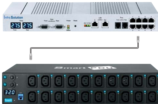
( Connecting SmartPDU to the expansion ports of InfraBox840 via Cat5/6 cable, Max. 8 PDUs per InfraBox )
