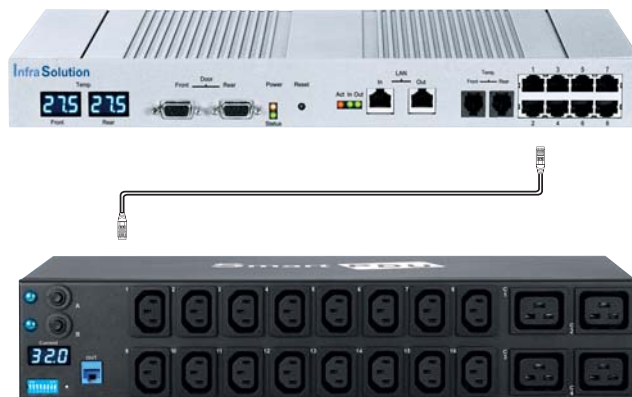
( Connecting SmartPDU to the expansion ports of InfraBox840 via Cat5/6 cable, Max. 8 PDUs per InfraBox )
